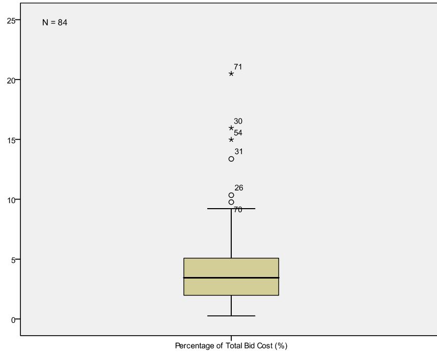
Fig. B- 41. Box plot for percentage of total bid cost for quality control before processing
